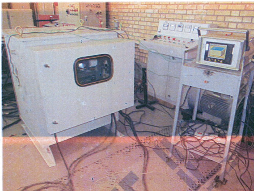
Figure 3. Temperature rise test
