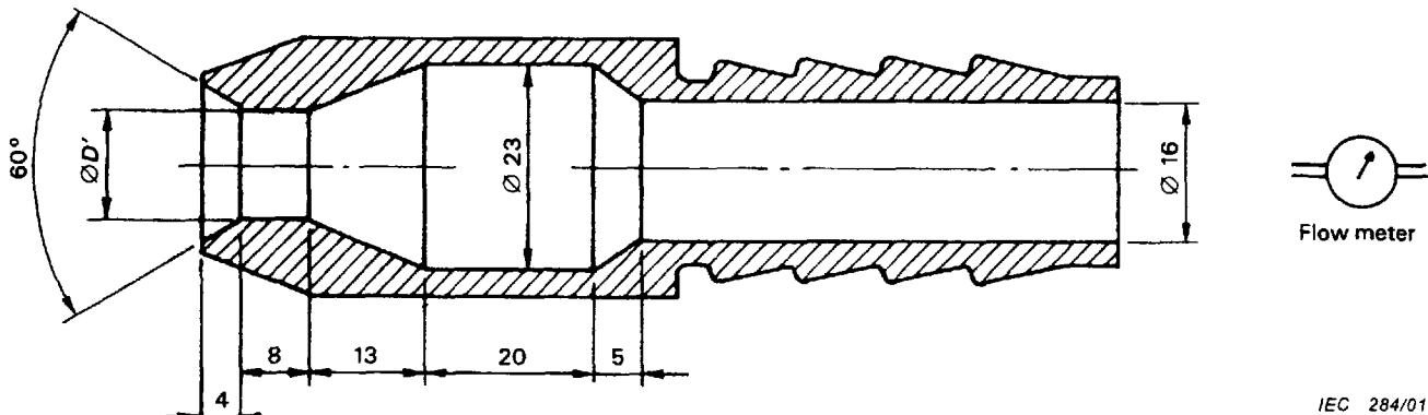
**Figure 6 – Test device to verify protection against water jets (hose nozzle)**
