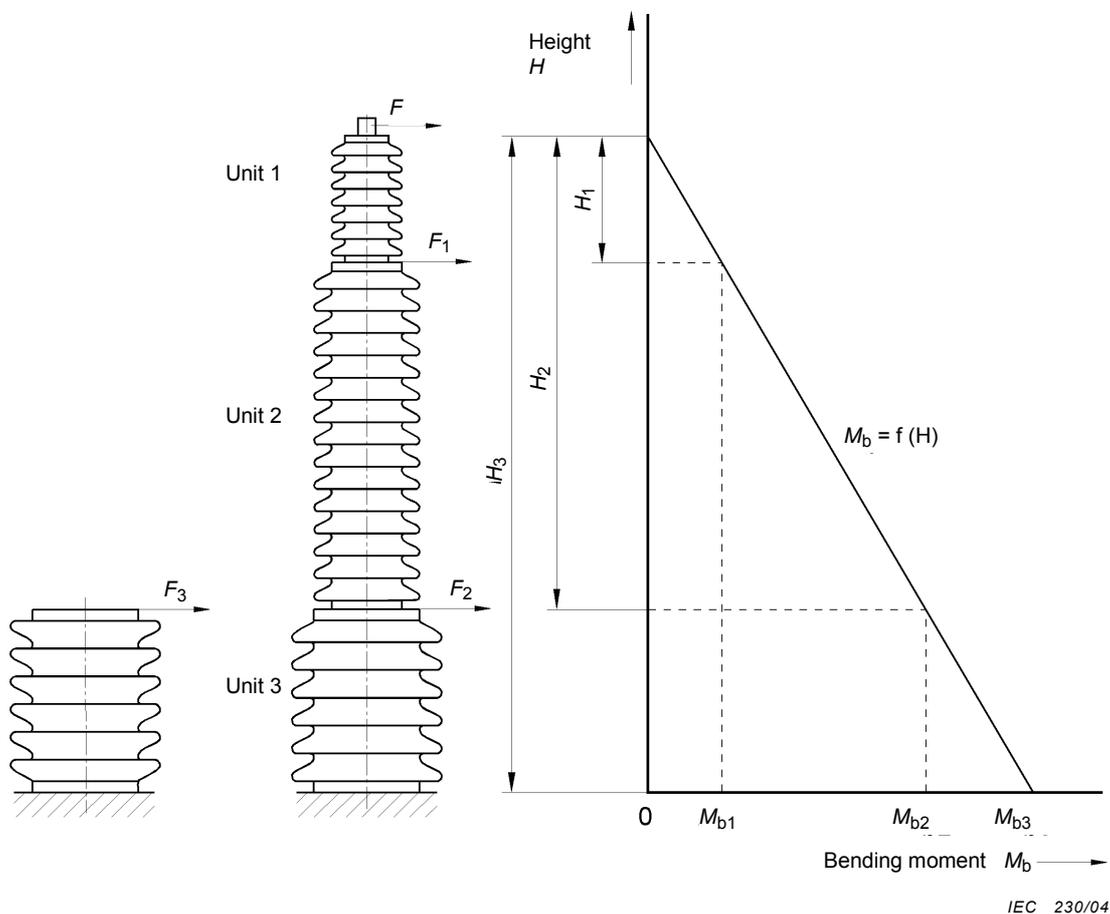
**Figure M.1 – Bending moment – multi-unit surge arrester**
