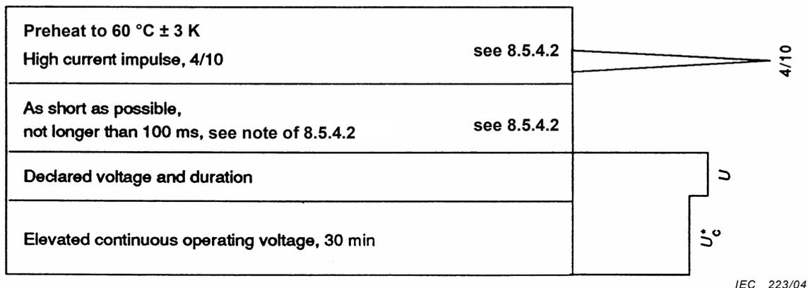
**Figure D.1 – Test on 10 000 A line discharge class 1,
