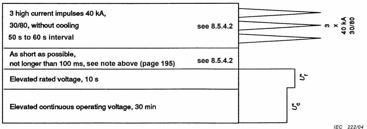
Figure C.2 – Thermal stability test on 20 000 A high lightning duty arresters (see 9.2.2)
