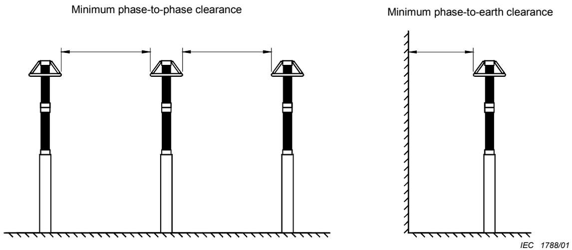
Figure L.1 – Typical three-phase arrester installation
