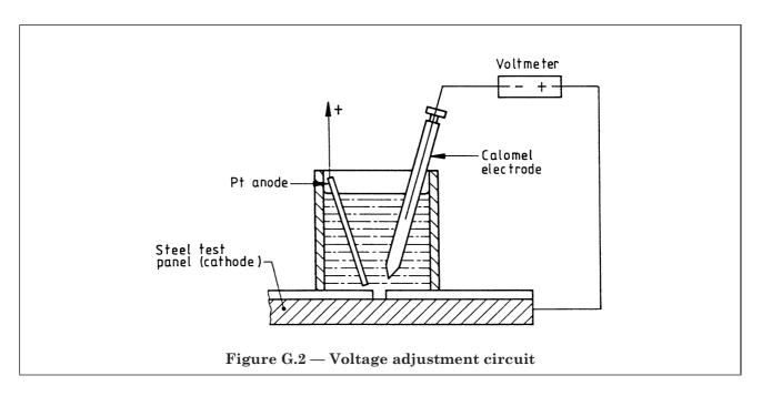
At intervals of 24 h record the voltmeter reading and adjust the variable resistor to correct any drift from the -1.500 V setting.
