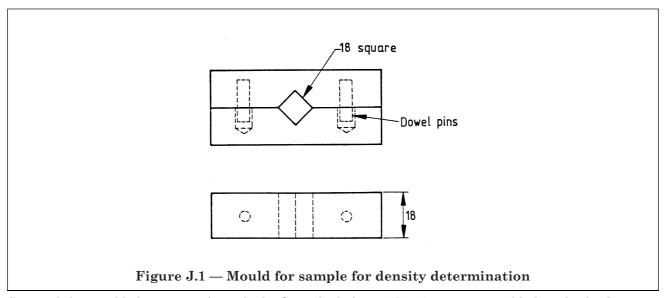
Suspend the moulded specimen from the hook on the balance (J.2.3) using a suitable length of nylon thread, and weigh it to the nearest milligram.
