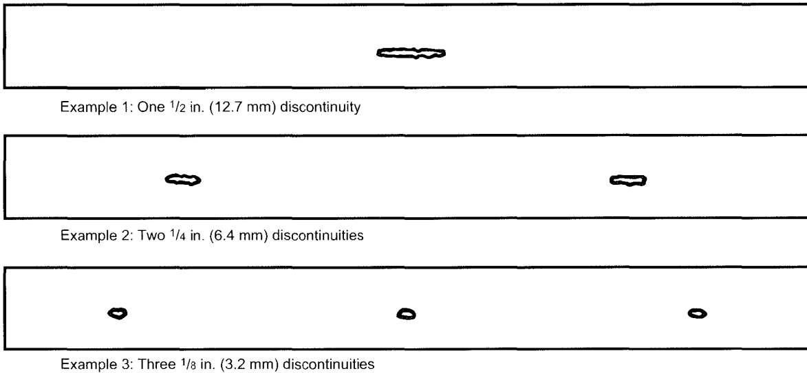
Figure 8—Examples of Maximum Distribution Patterns of Indicated Elongated Slag-inclusion-type Discontinuities
